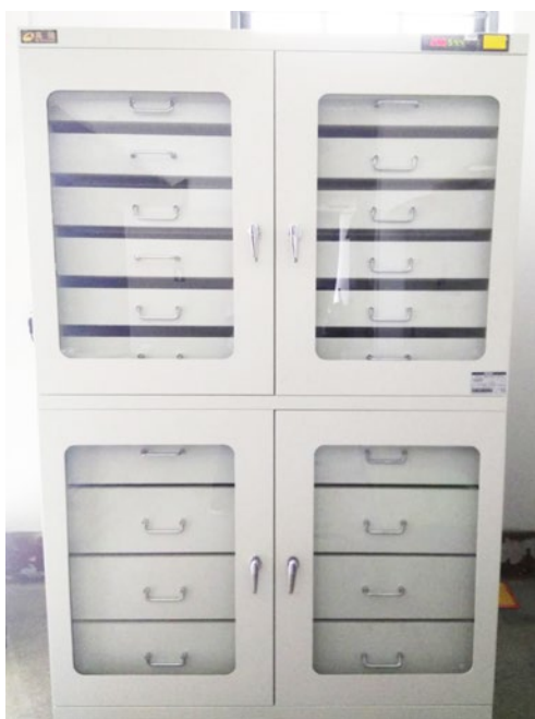
保管华侨纸质文物的恒温恒湿柜 Constant temperature and humidity cabinet for the preservation of overseas Chinese paper cultural relics
